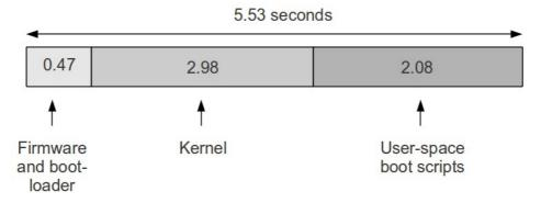
Now the boot time is of the order of 5 seconds, a 6 fold reduction on the initial configuration.
